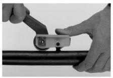
For longitudinal cutting of uncut cable, position the tool and press down the handle. The knife slides through the cable sheath, supported by the footed segment.
